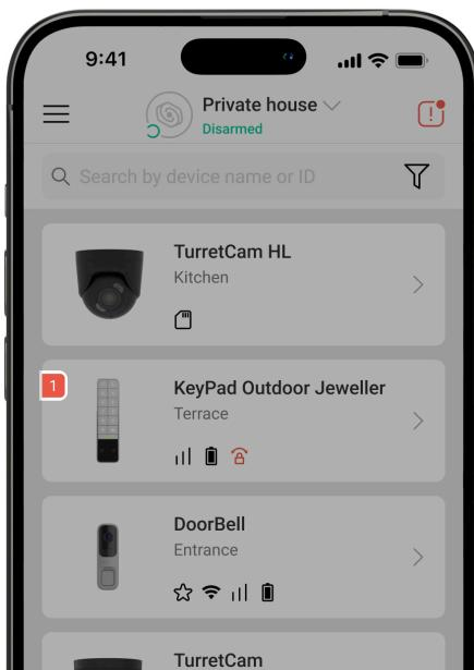
When the device detects a malfunction (for example, there is no connection via the Jeweller protocol), a malfunction counter is displayed in the Ajax app in the upper left corner of the device icon.
