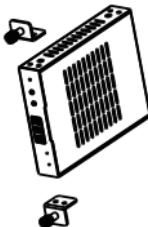
**Step 2:** Insert the product with mounting ears into a 4U rack (up to 12 units can be installed vertically), as shown in the figure below:
