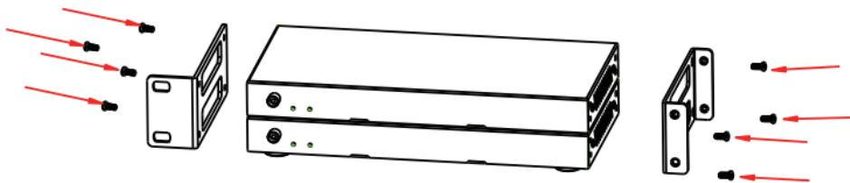
**Step 2:** Fix two 1U rack panels on another two stacked products in the same way, then use screws to fix two 1U rack panels together, as shown in the figure below:
